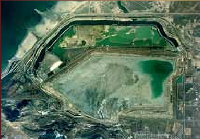
Figure 1. Kennecott Bingham Canyon Mine in Utah. (Left) Tailings impoundment (roughly 9,000 acres) with the Great Salt Lake at the top left. The pit is 0.75 miles deep, 2.5 miles wide, and covers 1,900 acres. (Right) Tailings are shown in the foreground (grey) with Salt Lake City in the background. Operations produced a 60 square-mile groundwater plume under valley to right, mostly from waste rock seepage. As of 2006, Kennecott had spent $370 million on cleanup and source control, and will be required to pump and treat aquifer water for at least the next 40 years. By 2009, 2.7 billion gallons of water will be treated annually to supply homes unable to use the aquifer.
