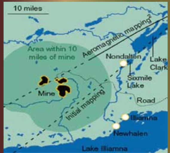
Figure 4. Geophysical locations of Lake Clark fault. Initial mapping of the Lake Clark fault estimates the fault to be within 10 miles. Aeromagnetic methods shows the fault a few miles to the north of the mine. In either case the fault is likely closer than 18 miles, the distance PLP assumes in its hazard calculations. Actual mapping of fault ———— Extrapolation of mapping - - - - -
