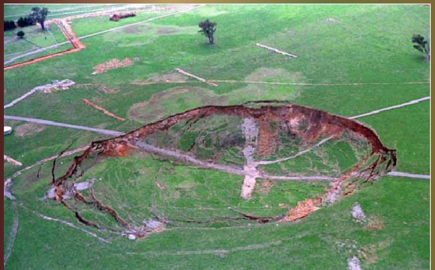
Figure 4. Subsidence due to block caving at the Ridgeway Mine, South Carolina from Newcrest Ltd. Cadia Operations, available at <http://en.wikipedia.org/wiki/Image:Elura.png#file>
