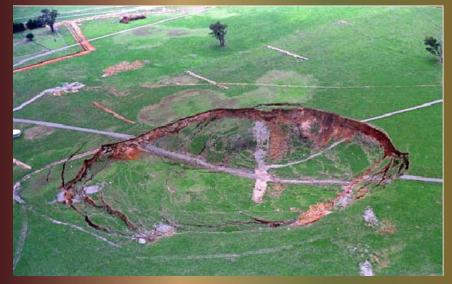
Figure 4. Subsidence due to block caving at the Ridgeway Mine, South Carolina from Newcrest Ltd. Cadia Operations, available at http://en.wikipedia.org/wiki/Image:Elura.png#file
