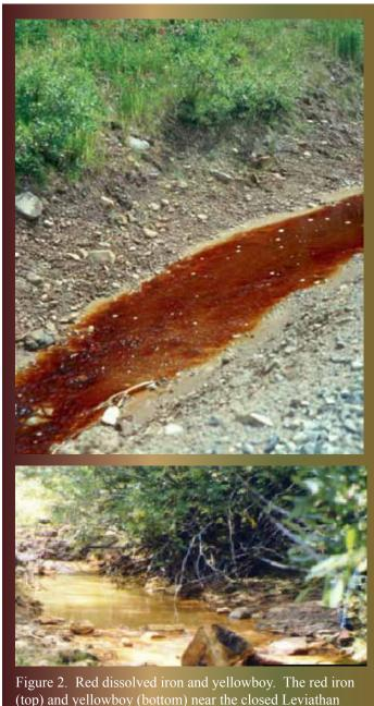
Figure 2. Red dissolved iron and yellowboy. The red iron (top) and yellowboy (bottom) near the closed Leviathan copper mine in California. Top photo G. Miller. Bottom photo Lahontan Regional Water Quality Board.
